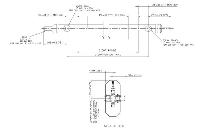
Figure 1.3 - High pressure water column (210 bar, 3045psi and 300 bar, 4350psi)
